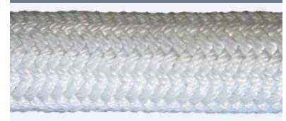
PANFLEX® PLUS is a double braid construction made of a 100% high tenacity polyamide core and ultra wear-resistant polyester cover. This construction endows ropes with the advantage of high strength, excellent wear resistance, and good shock absorption.
