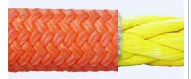
PANMAX® PLUS is the high-end jacketed rope composed of a construction of an independent 12-strand PANMAX® core and high tenacity sheath of polyester. This double-braided rope has higher strength, greater abrasion and UV resistance, lower stretch and creep than PANMAX®, which makes it ideal for all kinds of mooring applications.
