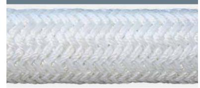
PANLINE® PLUS is constructed with a lightweight and highperformance multifilament polypropylene core and super strength and wear-resistant polyester cover. It outperforms nonjacketed ropes on UV & abrasion resistance and service life.
